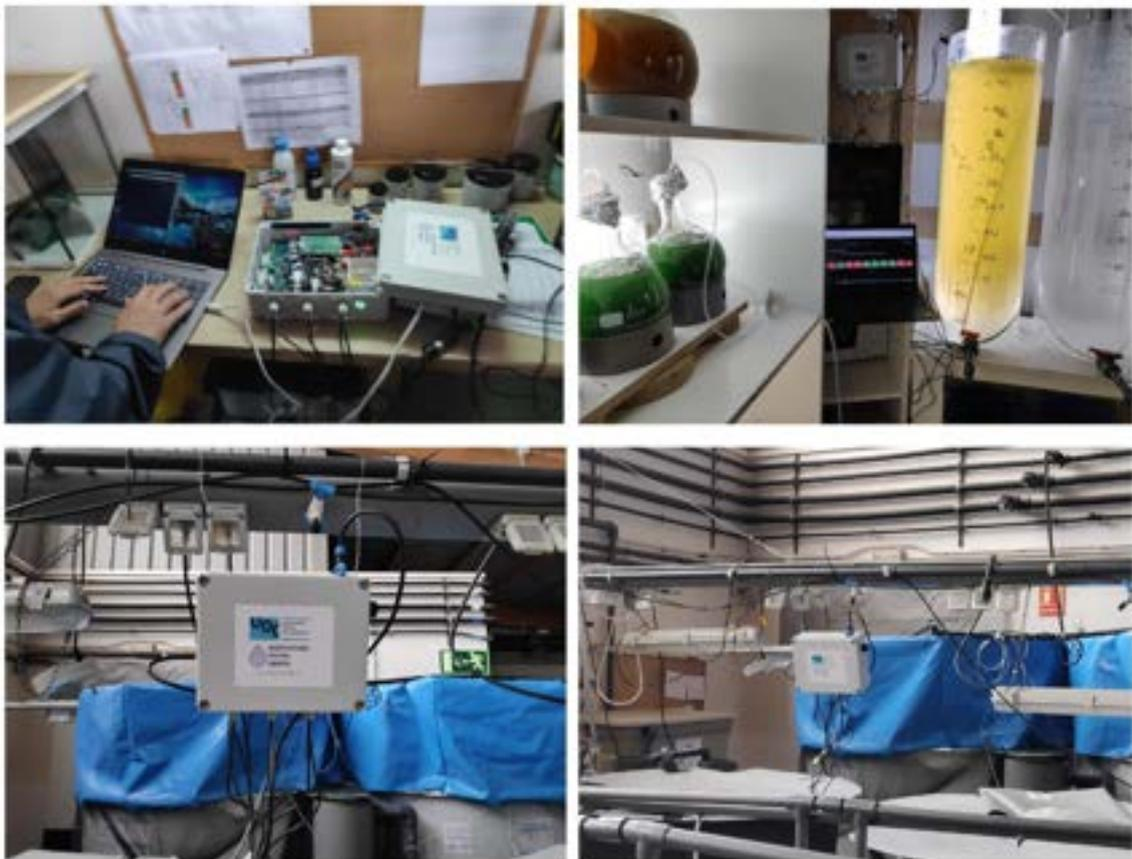
**Fig. 9.** Deployment of the ADO system in the Aquaculture Center in the Ebre's Delta. Device testing (top-left and right) and nodes installed in final positions (top-right, bottom-left and right).
