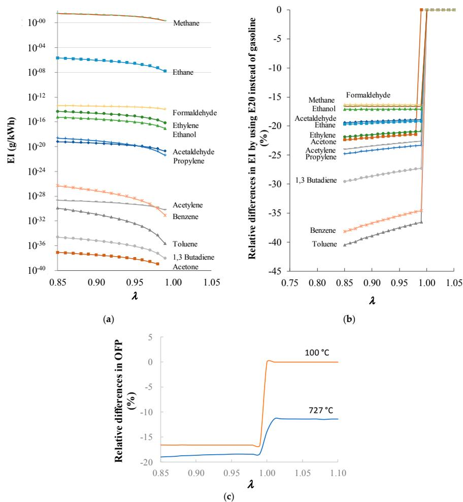
**Figure 9.** (a) Estimated emission indexes for the most relevant volatile organic compounds (VOCs) for gasoline and E20 fueled vehicles. Relative differences of using E20 instead of gasoline in (b) emission indexes and (c) ozone formation potential.
