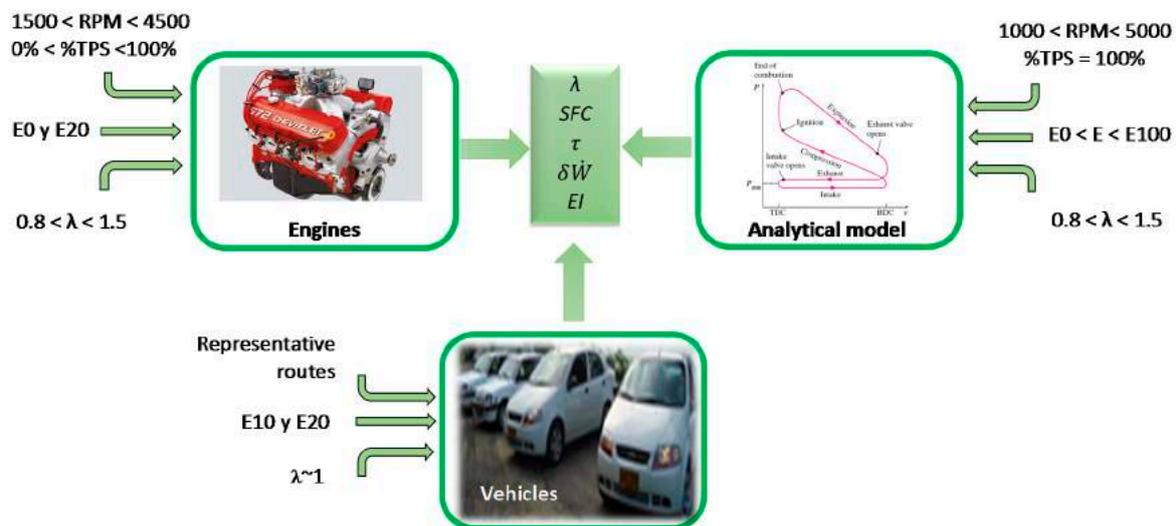
**Figure 1.** Illustration of the general methodology used to evaluate the effects of using ethanol-gasoline blends on the mechanical, energy and environmental performance of in-use vehicles during their useful life of operation.
