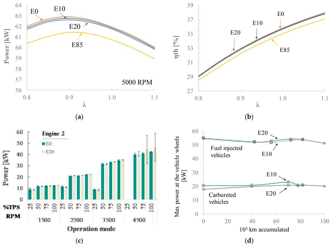
**Figure 2.** Power generated by engines when they operate with ethanol-gasoline blends. (a) Estimated power at 5000 RPM and (b) Estimated thermal efficiency displayed by engine 2 as a function of  $\lambda$  and ethanol content in the fuel; (c) Measured power delivered by engine 2 under steady-state conditions and different modes of operation; (d) Measured maximum power delivered by carbureted vehicles and fuel-injected vehicles after each ~10,000 km of operation.
