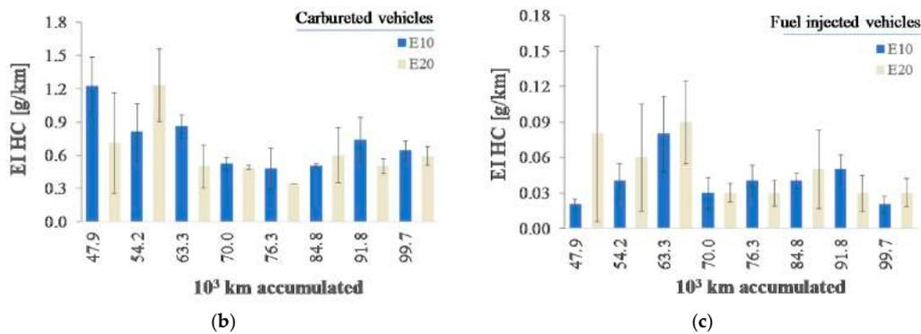
**Figure 8.** HC emission indexes obtained from (a) Our analytical model for engines; (b) Carbureted and (c) Fuel-injected vehicles following the NEDC on a chassis dynamometer every 10,000 km of operation.
