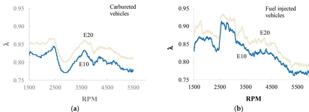
**Figure 4.** Effect of fuel changes in the operational conditions under which the vehicles work.  $\lambda$  vs. RPM obtained from (a) carbureted and (b) fuel-injected vehicles at full load.
