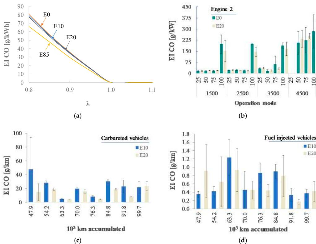
**Figure 6.** CO emission indexes obtained by: (a) Our analytical model for engines; (b) Engine tests under steady-state condition; (c) Carbureted and (d) Fuel-injected vehicles following the NEDC on chassis dynamometers, after every 10,000 km traveled.
