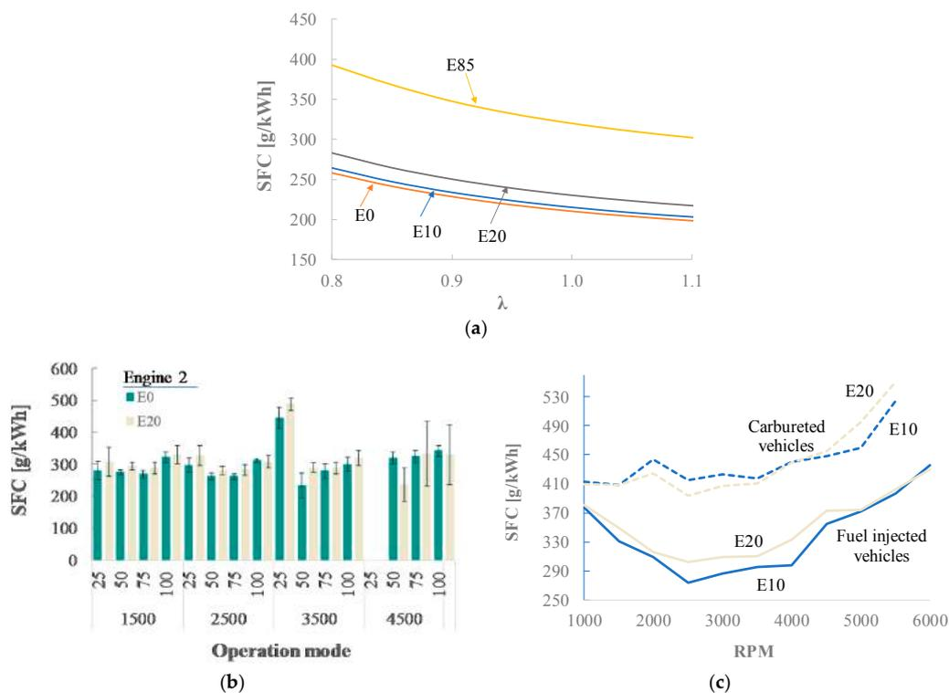
**Figure 3.** Results of specific fuel consumption (SFC) obtained: (a) analytically; (b) testing engine 2 under steady-state conditions; and (c) carbureted and fuel-injected vehicles under steady-state conditions at full load on the chassis dynamometer after 72,000 km of operation.
