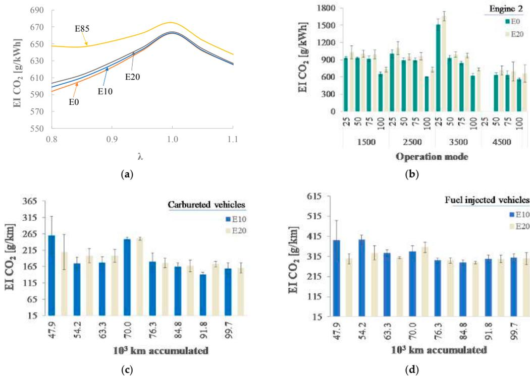
**Figure 5.** CO<sub>2</sub> emission indexes obtained through: (a) Analytical model; (b) Engine tests under steady-state conditions; (c) Carbureted and (d) Fuel-injected vehicles, following the new European driving cycle (NEDC) on chassis dynamometers, after every 10,000 km traveled.
