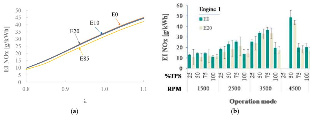
**Figure 7.** NOx emission indexes obtained by (a) Our analytical model for engines; and (b) Tests on engine 1 under steady-state conditions, when the engine used different ethanol-gasoline blends.
